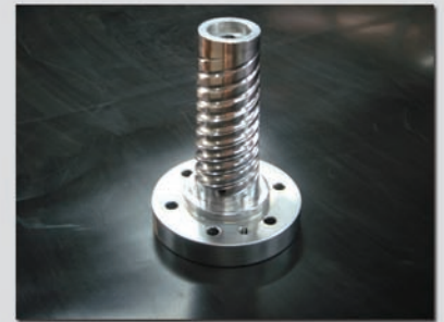
Optimized die design ensures uniform flow distribution.
