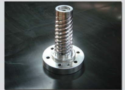
Optimized die design ensures uniform flow distribution.
