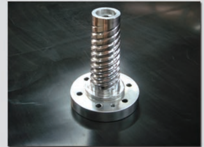
Optimized die design ensures uniform flow distribution.
